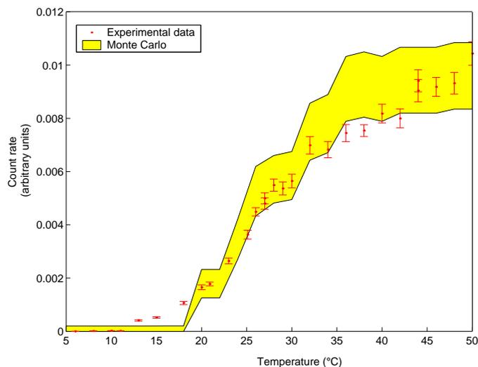
**Figure 2.** Detector response (count rate) of the 1l SBD-1000 spiked with 20 Bqs of  $^{241}\text{Am}$  as a function of temperature. A critical length of  $L=18R_c$  is necessary to fit the data.
